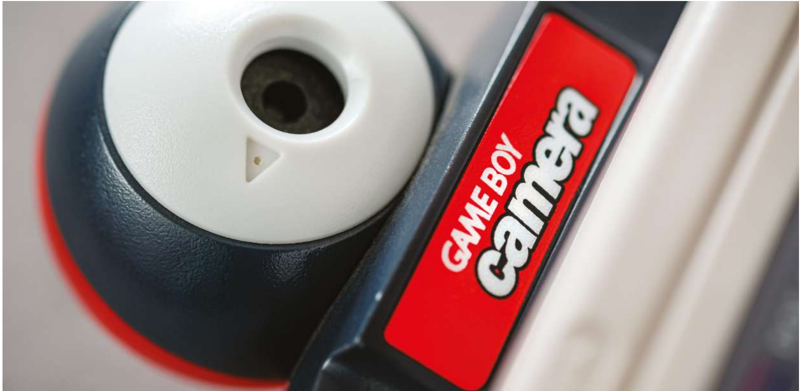
Sporting a 128 × 128-pixel CMOS sensor, the Game Boy Camera is capable of snapping grayscale images using the four-colour palette of the Game Boy.
